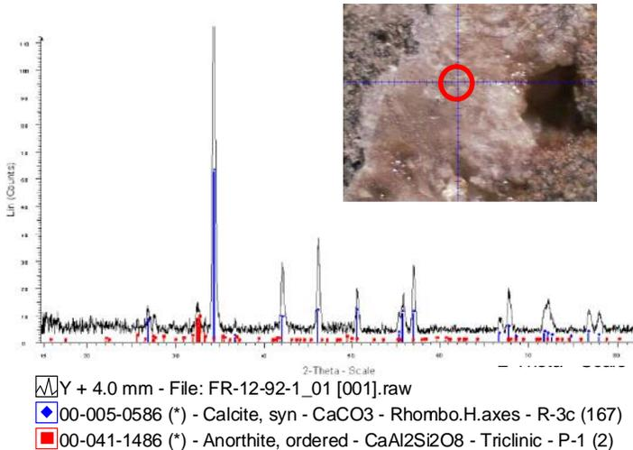
**Figure 2:**  $\mu$ XRD data of a volcanic tuff obtained using a Bruker D8 Discover diffractometer. Inset: micrograph of spot analyzed showing 100  $\mu$ m diameter spot analyzed in red.
