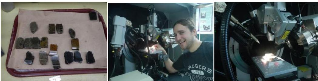
**Figure 3:** *Left* - Rock slabs cut from samples collected in Oregon being adhered to glass with epoxy resin in the petrographic thin sectioning lab at Brock University. *Center* - Placing tuff sample slabs into the Micro X-Ray Diffraction Instrument at the University of Western Ontario. *Right* - Bruker D8 Discover Diffractometer with General Area Detector Diffraction System at the University of Western Ontario.
